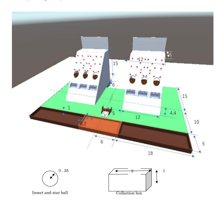
Fig. 2 Dimensions of contest field. (unit is 100mm)
