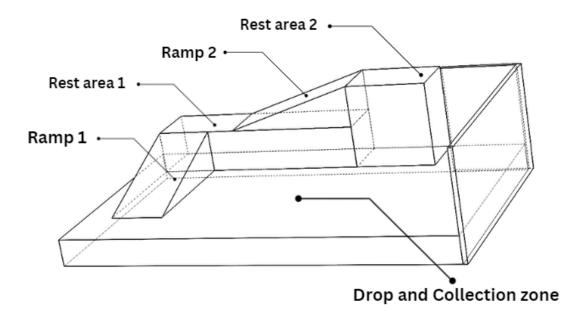
**Ramp 1** – Designed with care, the 18-degree ramp offers a smooth climb for the mobile robots crafted by participants. This gently sloped ramp leads directly to a rest area, making it easy for robots to move safely and efficiently throughout the competition space. This thoughtful design ensures the robots can perform at their best while navigating seamlessly from one section to the next.
